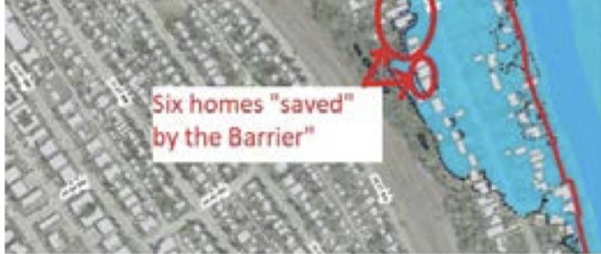
Groundwater Flooding in North Bowness with Barrier
